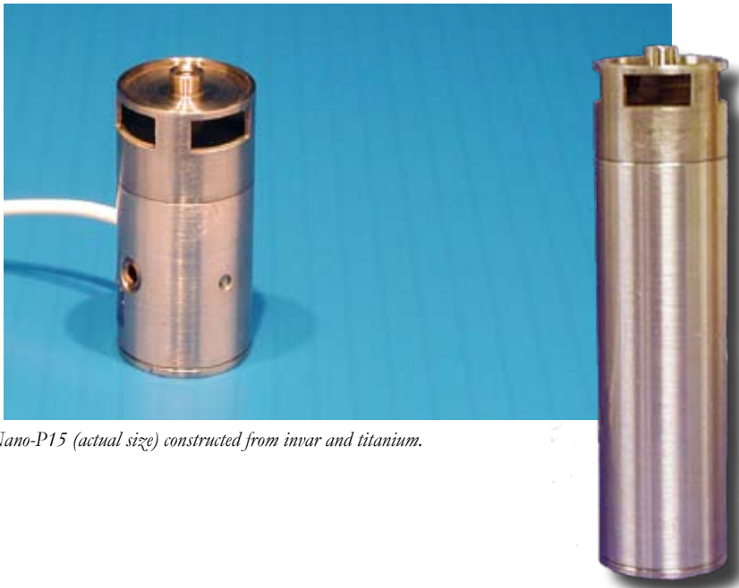
Nano-P70 (actual size) constructed from invar and titanium.
