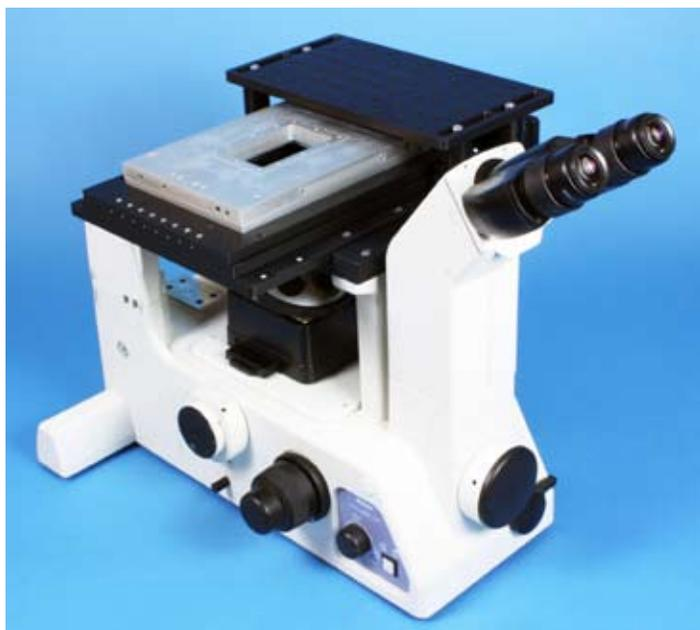
Nano-View® 300-3 mounted on a Nikon inverted microscope. Optional breadboard for mounting of probes and accessories is also shown.
